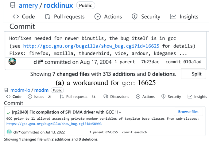
(a) a workaround for gcc 16625 (b) a workaround for gcc 58993 Fig. 7: The C++ bugs
