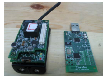
Figure 5. Mobile badge (MicaZ) and beacon node (Taroko).
