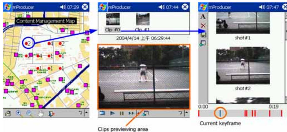
Figure 9: mProducer user interface showing the location-based content management (left screen), material pool (middle screen), and storyboard interface (right)
