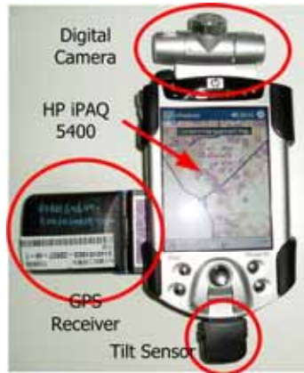
Figure 2: HP iPAQ 5450 with a digital camera, a GPS receiver and a tilt sensor
