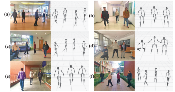
Figure 14: Multi-user 3D posture tracking in different environments.
