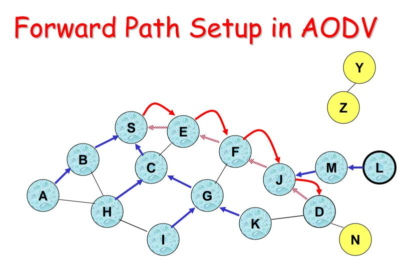
Forward links are setup when RREP travels along the reverse path
