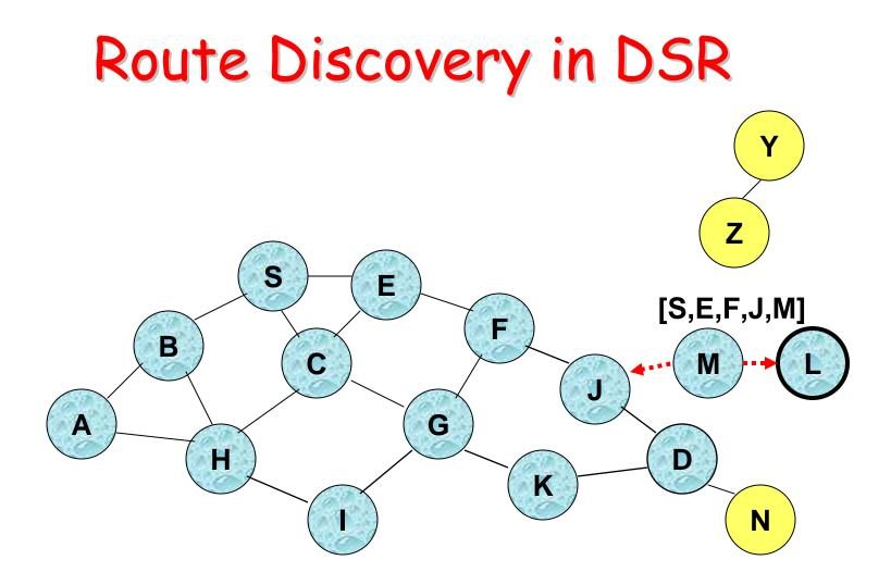
• Node D does not forward RREQ, because node D is the intended target of the route discovery
