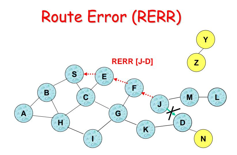
J sends a route error to S along route J-F-E-S when its attempt to forward the data packet S (with route SEFJD) on J-D fails
