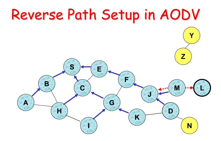
• Node D does not forward RREQ, because node D is the intended target of the RREQ
