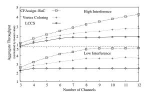
Fig. 7. Comparison of application throughput for CBR/UDP fbws for the three algorithms.
