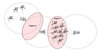
Fig. 1. Channel assignment should be based on user performance. The unshaded circles indicate the interference radius of each AP.
