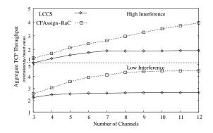
Fig. 8. Comparison of application throughput for FTP/TCP fbws for the three algorithms.
