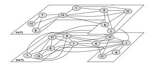
Fig. 15. Visualization of the testbed over two (out of the four) fbors. LCCS based channel assignment shown in circles representing AP positions. Edges indicate overlap in coverage.
