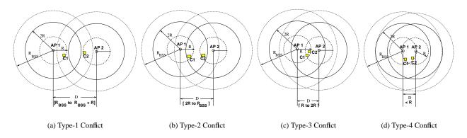
Fig. 3. Figure shows four different *conflict* situations that can arise with two APs. Shown for each AP is its communication radius (R) and a region of radius 2R where transmissions from associated clients would interfere.
