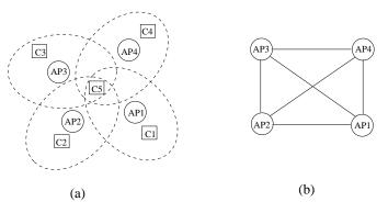
Fig. 5. (a) A WLAN example and (b) the graph created by the vertex coloring formulation.
