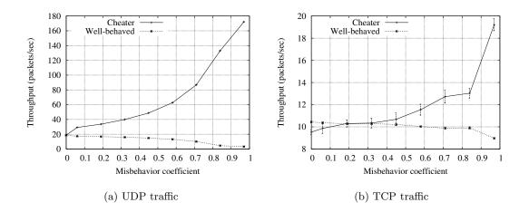
Figure 6: Throughput comparison between misbehaving and well-behaved stations.
