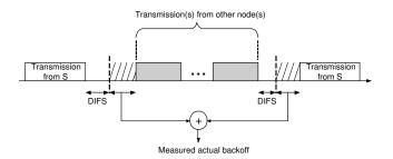
Figure 3: Measurement of the actual backoff. Transmissions from S are interleaved with one or more transmissions from other nodes (including the AP). The transmission includes in addition to the DATA frame all the control frames, such as RTS, CTS, and ACK, as well as the interleaving idle periods of SIFS. The measured value is the sum of all idle intervals (not including interframe spaces) between two transmissions from S.
