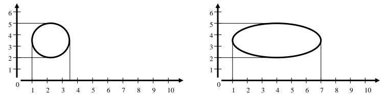
Scaled by a factor of 2 in the x direction and not scaled in the y direction. Width changes from 3.5 to 7.
