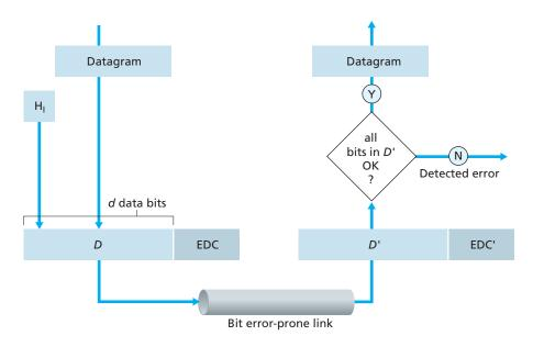
Figure 5.3 • Error-detection and -correction scenario
