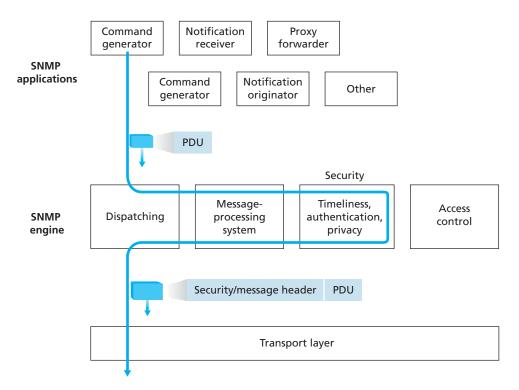
Figure 9.5 • SNMPv3 engine and applications
