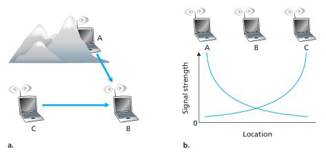
Figure 6.4 Hidden terminal problem caused by obstacle (a) and fading (b)
