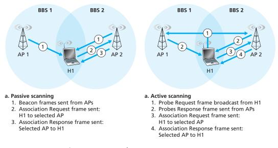
Figure 6.9 • Active and passive scanning for access points
