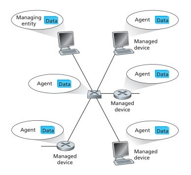
Figure 9.2 • Principal components of a network management architecture
