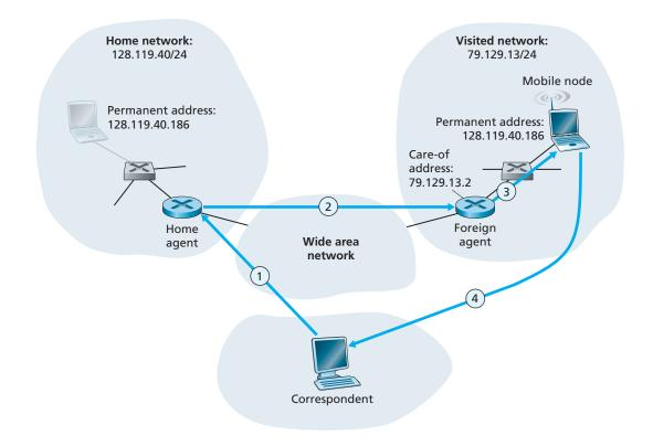
Figure 6.23 • Indirect routing to a mobile node
