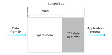
Figure 3.38 The receive window (rwnd) and the receive buffer
