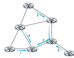
a. Stepwise construction of spanning tree
