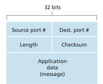
Figure 3.7 • UDP segment structure
