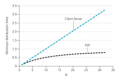
Figure 2.25 • Distribution time for P2P and client-server architectures
