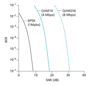
Figure 6.3 • Bit error rate, transmission rate, and SNR
