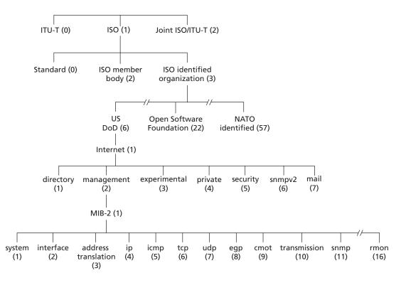
Figure 9.3 • ASN.1 object identifier tree
