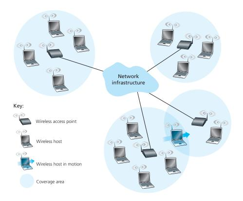
Figure 6.1 Elements of a wireless network
