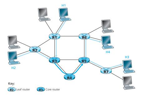
Figure 7.25 • A simple Diffserv network example
