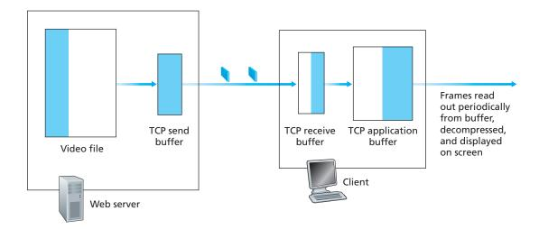
Figure 7.2 • Streaming stored video over HTTP/TCP
