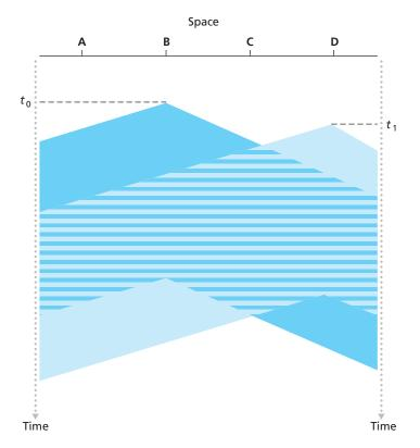
Figure 5.12 • Space-time diagram of two CSMA nodes with colliding transmissions
