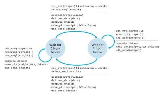
Figure 3.57 • An incorrect receiver for protocol rdt 2.1
