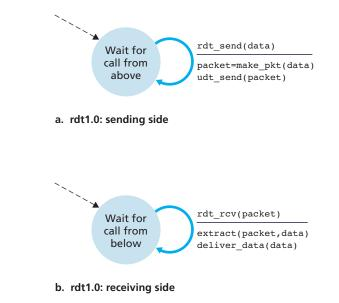
Figure 3.9 < rdt1.0 - A protocol for a completely reliable channel
