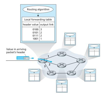
Figure 4.2 • Routing algorithms determine values in forwarding tables
