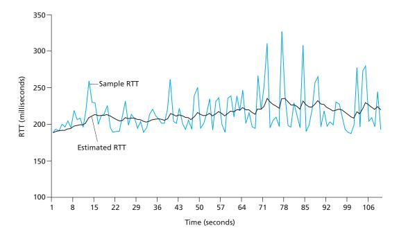
Figure 3.32 • RTT samples and RTT estimates
