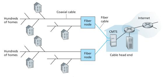
Figure 1.6 A hybrid fiber-coaxial access network
