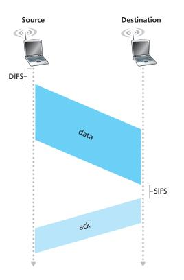
Figure 6.10 • 802.11 uses link-layer acknowledgments
