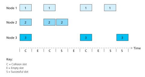
Figure 5.10 A Nodes 1, 2, and 3 collide in the first slot. Node 2 finally succeeds in the fourth slot, node 1 in the eighth slot, and node 3 in the ninth slot
