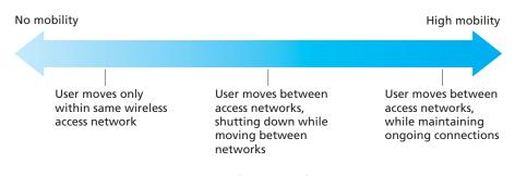
Figure 6.21 • Various degrees of mobility, from the network layer's point of view
