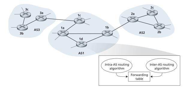
Figure 4.32 • An example of interconnected autonomous systems
