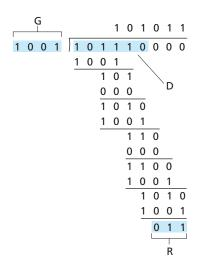
Figure 5.7 • A sample CRC calculation
