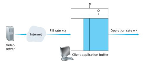
Figure 7.3 Analysis of client-side buffering for video streaming
