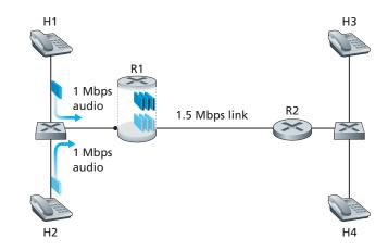
Figure 7.27 ♦ Two competing audio applications overloading the R1-to-R2 link
