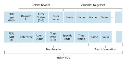
Figure 9.4 SNMP PDU format
