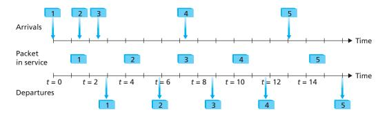
**Figure 7.18** The FIFO queue in operation
