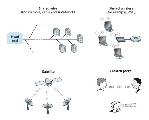
Figure 5.8 • Various multiple access channels
