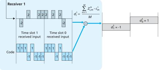
Figure 6.6 • A two-sender CDMA example
