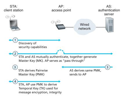
Figure 8.31 • 802.11i: four phases of operation
