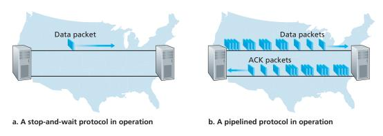
Figure 3.17 • Stop-and-wait versus pipelined protocol
