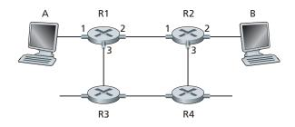
Figure 4.3 • A simple virtual circuit network
