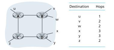
Figure 4.34 • Number of hops from source router A to various subnets
