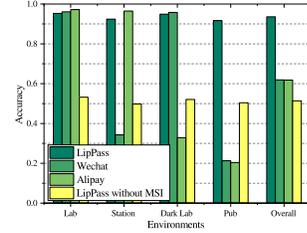
Fig. 14. Authentication accuracy of *LipPass*, Wechat, Alipay and *LipPass* without mouth state identification (MSI).
