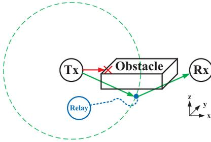
Fig. 1. It is common in mmWave communication that the transmission from a transmitter (Tx) to a receiver (Rx) is blocked by an obstacle.
