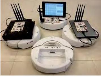
Fig. 2. Prototype of mobile relay.
