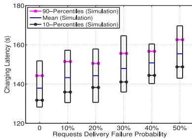
Fig. 18. Charging latency with delivery failure ratio of charging requests.
