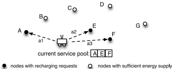
Fig. 3. On-demand charging of nodes:  $a_1$ ,  $a_2$ , and  $a_3$  represent the corresponding distances to requesting nodes.
