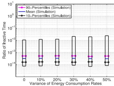
Fig. 17. Inactive time ratio with energy consumption variance.
