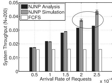
Fig. 9. System throughput with 200 nodes.
