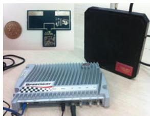
Fig. 1. Lab settings for WISP-based charging.
