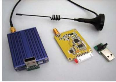
(b) The device of EE radio. The left box contains the actual chipset on the right side.
