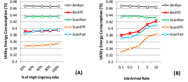
Figure 5: The utility energy consumption vs. % of HU and job arrival rate for the five scheduling schemes
