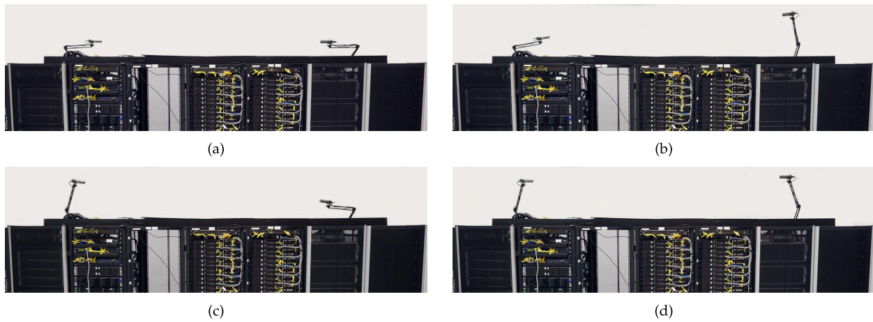
Fig. 4. Deployment of a pair of liftable 3D Beamforming radios onto 2 different layers. (a) Case 1: Both of the radios are on the lower layer. (b) Case 2: The right radio is higher than the left one. (c) Case 3: The right radio is lower than the left one. (d) Case 4: Both of radios are on the higher layer.
