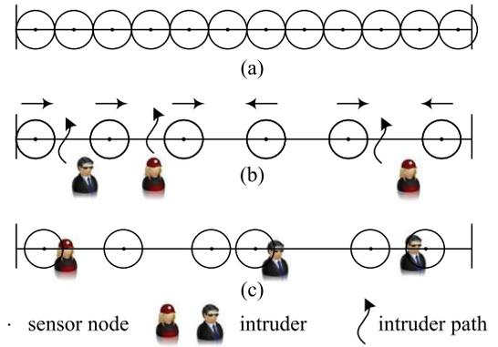
Fig. 3. (a) Full barrier coverage by static sensors; (b) and (c) Barrier coverage by mobile sensors [62].
