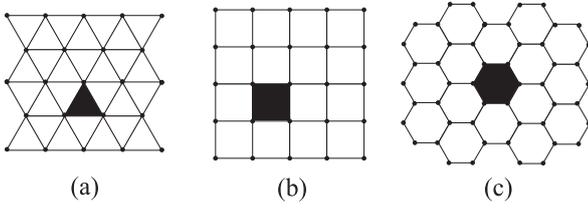
Fig. 7. Grid sensor deployment using (a) triangle, (b) square, and (c) hexagon pattern.
