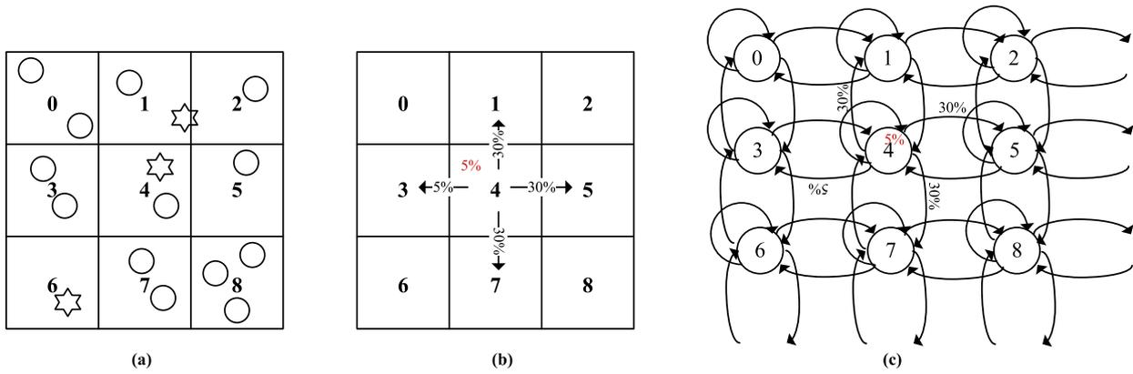
Fig. 18. Illustration for random walk for mobile sensors [114].
