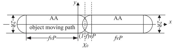
Fig. 14. The active area in the synchronized schedule when  $R$  is large [169].
