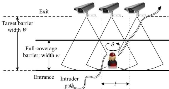
Fig. 10. Concept of local face-view camera barrier coverage [94].
