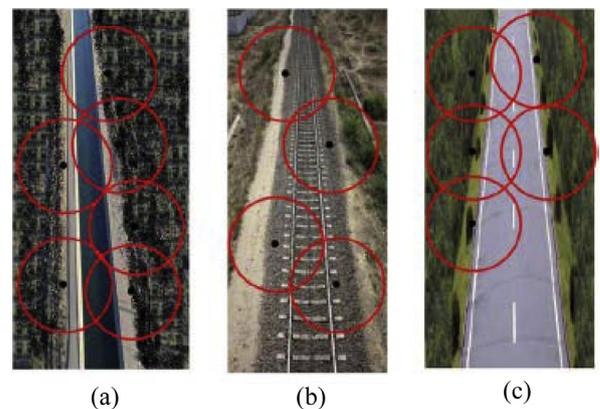
Fig. 12. Examples of the coverage of Field of Interest (FoI) with sensors deployed outside the edges. (a)–(c) Sensors monitoring canal water surface, railway track, and road surface, respectively [116].
