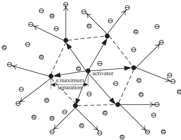
Fig. 15. A simplification of the node activation process in PCP. Activated nodes try to form a triangular lattice over the area [88].
