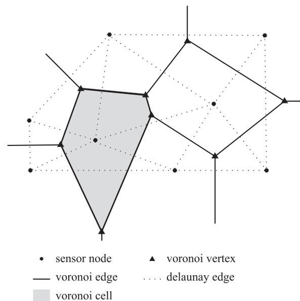
Fig. 2. Illustration of Voronoi diagram and Delaunay triangulation for 8 sensors [1].
