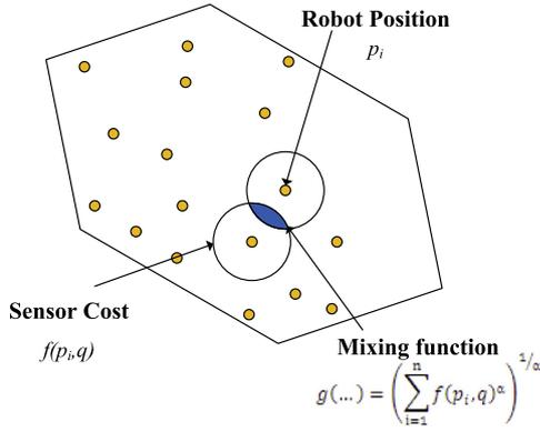
**Fig. 16.** The mixing function is illustrated in this figure. It determines how information from multiple robot sensors are combined, shown graphically as the intersection of the two circles in the figure [3].
