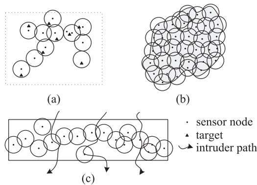
**Fig. 1.** Three kinds of typical coverage: (a) Target coverage. (b) Area coverage. (c) Barrier coverage.
