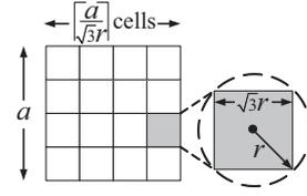
Fig. 4. Tessellation of the square into cells.
