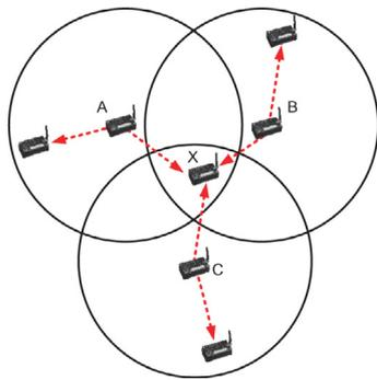
**Fig. 1.** An example of how the ND is conducted in MPR networks. Node A, B, and C are broadcasting their discovery messages simultaneously. Node X is in the coverage of all the three nodes. If they are in a SPR network, collision will occur at X. However if they are in a 3-MPR network, X will successfully receive three nodes' discovery messages simultaneously.
