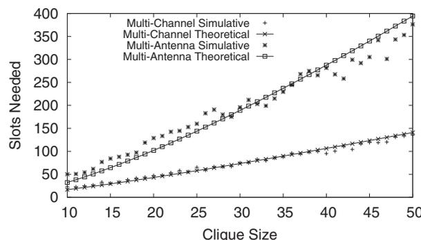
Fig. 15. Comparison between multi-antenna MPR and multi-channel MPR.
