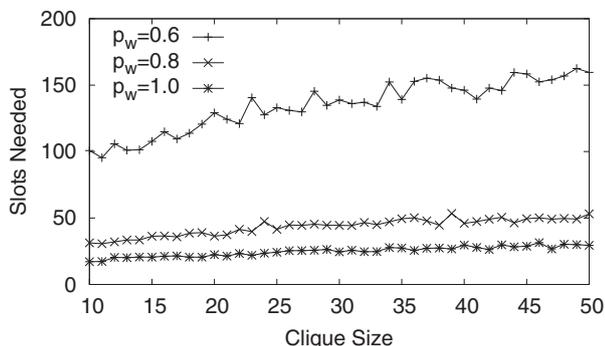
Fig. 13. Comparison of different duty cycles (idealized MPR).
