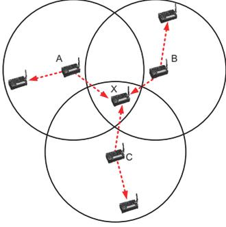
Figure 1. An example of how the ND is conducted in MPR networks. Node  $A$ ,  $B$ , and  $C$  are broadcasting their discovery messages simultaneously. Node  $X$  is in the coverage of all the three nodes. If they are in a SPR network, collision will occur at  $X$ . However if they are in a 3-MPR network,  $X$  will successfully receive three nodes' discovery messages simultaneously.
