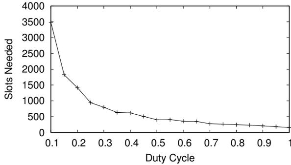
Figure 6. Comparison of Different Duty Cycles (ALOHA-like,  $n = 50$ )
