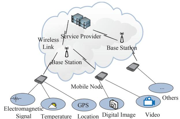
Fig. 1. The Architecture of Cloud-Based Participatory Sensing.
