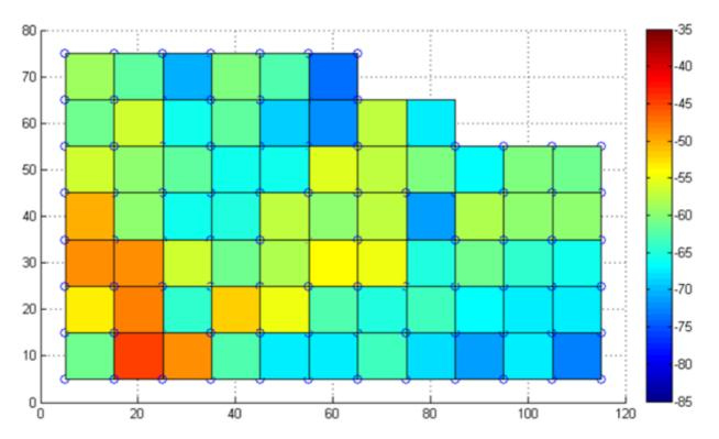
This is the radio map of one of the routers. We divide the whole space in to several blocks, as the picture shown. The color of each blocks indicates the RSS of the access point.
