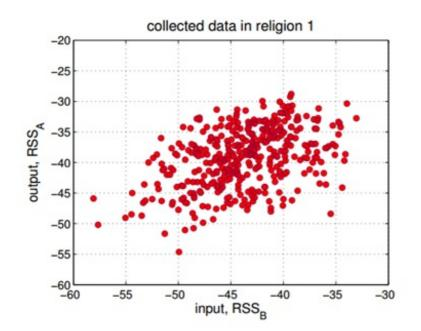
We suppose device A is the standard device. In this given location, device A and another device B all get the RSS from the same AP. We suppose that the RSSA is the standardvalue, and RSSB should be mapped to RSSA collected by device A. Then we use Gaussian Process to do the regression, illustrated by the following figure.
