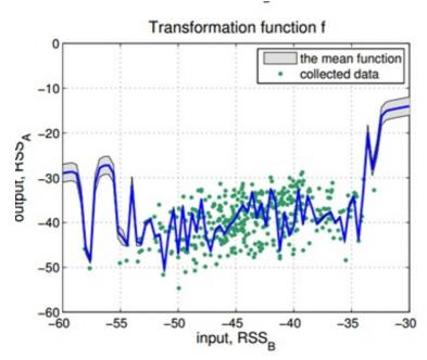
In this way, for a new input RSS value collected by device B we can map it to the standard device A.
