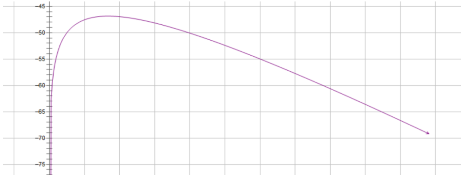
Fig. 4 Log attenuation model of RSSI
