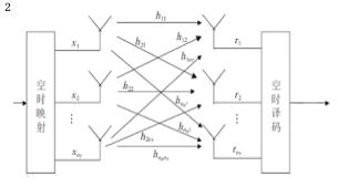
3. Space-multiplexing: At the transmitter, high-rate data streams are partitioned into multiple lower-rate sub-data streams, and different sub-streams are transmitted on different transmit antennas on the same frequency band. Space diversity: Use the multiple transmission paths provided by multiple antennas on the transmitting or receiving side to send the same data to enhance the transmission quality of the data.
