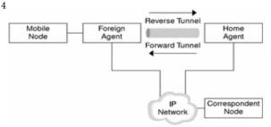
5. Registration process: Initiate: The MN sends a registration request to the FA. Then FA switches registration to the HA. HA will send reply to FA in order to check. Finally, the FA uses its registration and relay it to MN.
