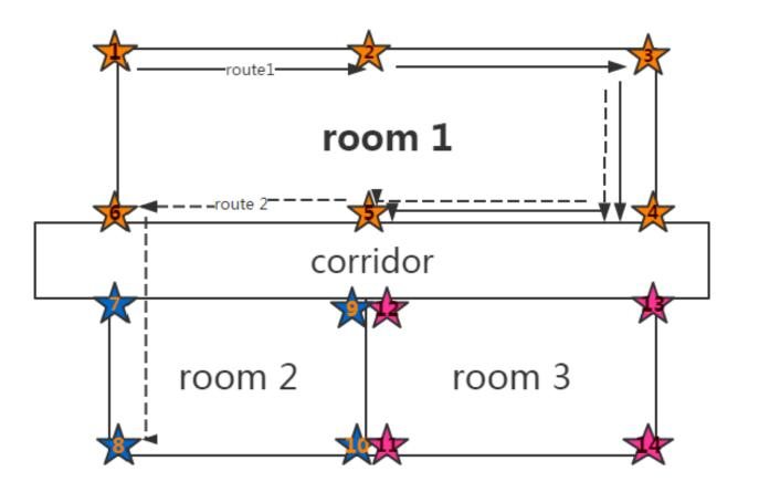
Sort out similar Anchors  $\downarrow$  Larger than 3 Anchor array A, Anchor array B  $\downarrow$ Find scaling factor k and rotation matrix  $\beta$  $\mathbf{A}^{T}(\mathbf{k}\beta)^{T} = \mathbf{B}^{T}$
