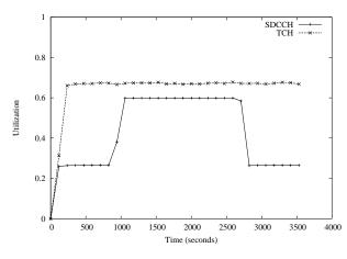
Figure 12: Channel utilization under SRP
