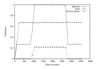
Figure 10: The simulated utilization for a sector implementing WRED. Notice that the queue occupancy stays low due to the decreased priority of Internet-originated messages.
