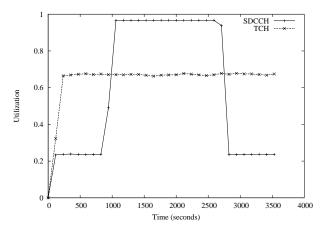
Figure 16: Channel utilization under DCA
