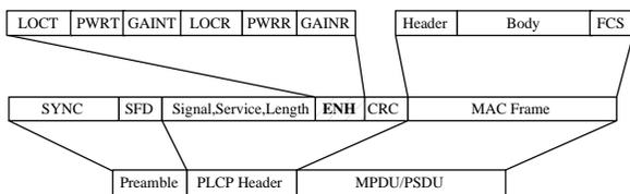
Fig. 8. Frame structure
