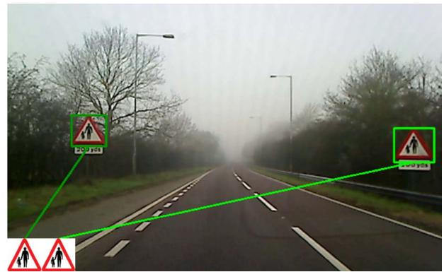
Fig. 16. Image that shows the detection of the “Pedestrians in Road” sign (taken from video 2).
