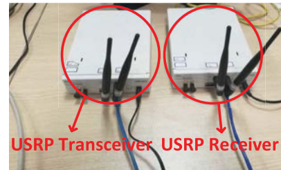
Fig. 13. Our testbed uses two USRPs as the ZigBee transceiver and receiver.
