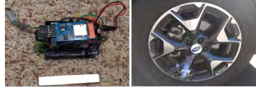
Fig. 26: Attach a Hall-based RPM sensor to the wheel.
