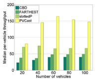
Fig. 4: Per-vehicle throughput (pkts/sec)
