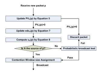
Fig. 3: PVCast's architecture. The figure shows the flow chart of PVCast.
