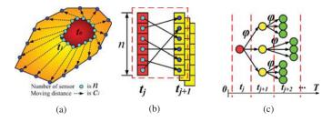
Fig. 4. (a) Sensors move to candidate positions on a convex hull from  $t_0$  to  $t_1$ . (b) Two consecutive stages MBC problem converts to a weighted bipartite matching problem. (c) A *K-D* MBC problem reduces to a multiple-stage weighted bipartite matching problem.
