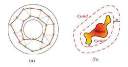
Fig. 2. (a) Coverage graph of the sensor network represented by Fig. 1(b). There are two vertex-disjoint cycles in the closed belt region. (b) Two cycles barrier cover a dynamic object. The interval between chain and object is  $\varepsilon$ . The interval between two cycles is m.
