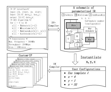
Figure 2: The synthesis of AES IP core
