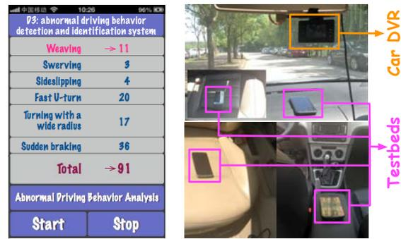
Fig. 7. User interface of  $D^3$  and testbeds.
