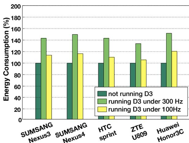
Fig. 16. Energy consumption on 5 types of devices with  $D^3$  under different sampling rates and without running  $D^3$ .
