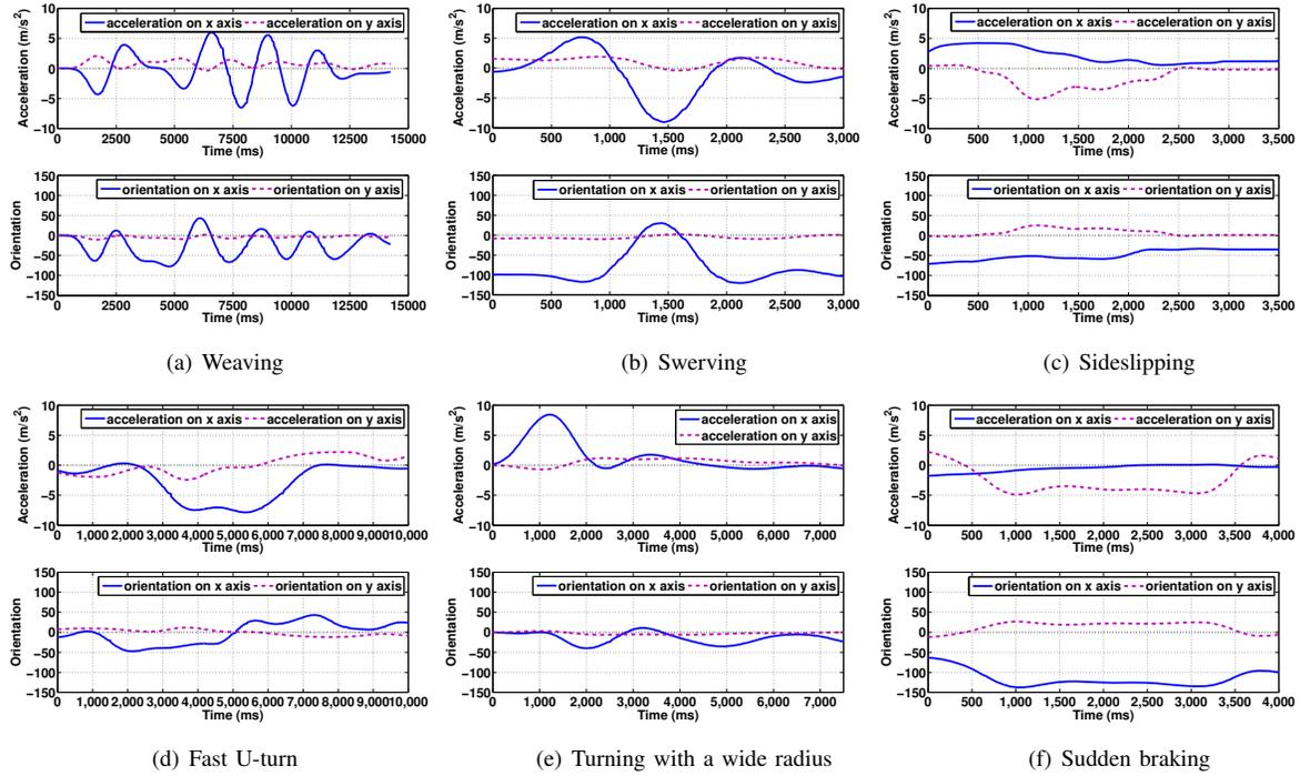
Fig. 3. The acceleration and orientation patterns of the six types of abnormal driving behaviors from an accelerometer and an orientation sensor's readings.
