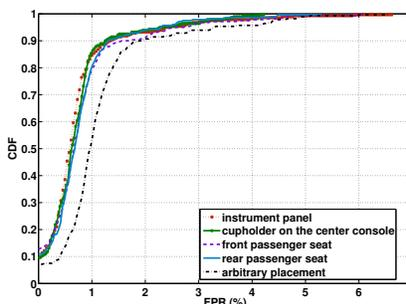
Fig. 13. CDF of FPR under different smartphone placements with SVM classifier model.
