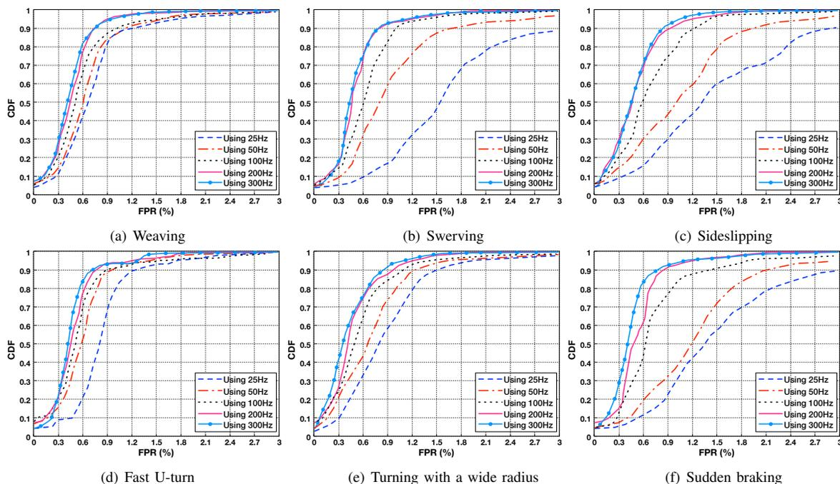
Fig. 15. CDF of FPR using different sampling rates for each type of abnormal driving behaviors.
