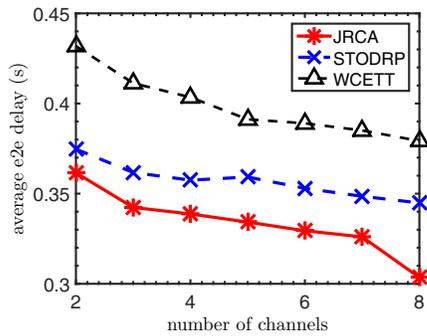
Fig. 4 E2e delay with the number of channels.
