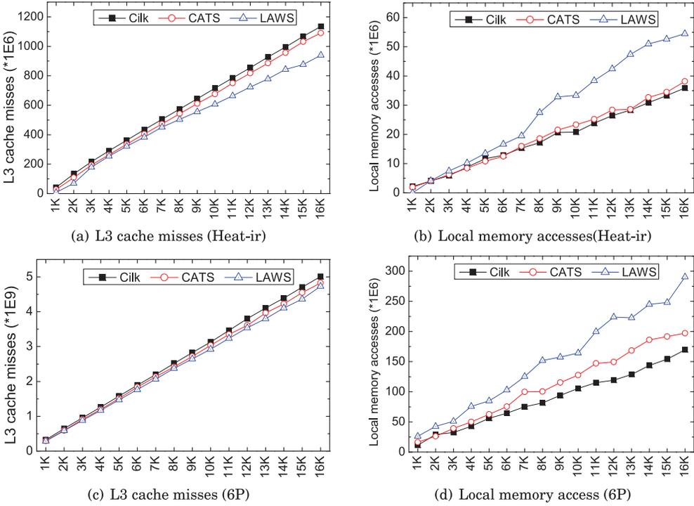
Fig. 11. L3 cache misses and local memory accesses of the straggler socket in Heat-ir and 6P on AMD server.
