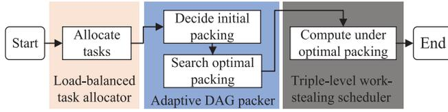
Fig. 3. The processing flow of an iterative D&C program in LAWS.
