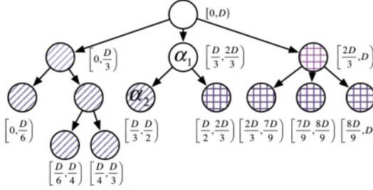
Fig. 4. Allocate the tasks to the two sockets of a dual-socket architecture.
