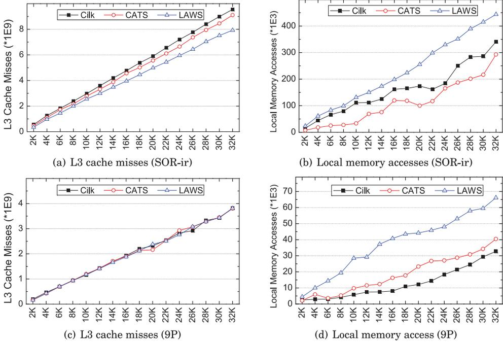
Fig. 12. L3 cache misses and local memory accesses of the straggler socket in SOR-ir and 9P on the Intel server.
