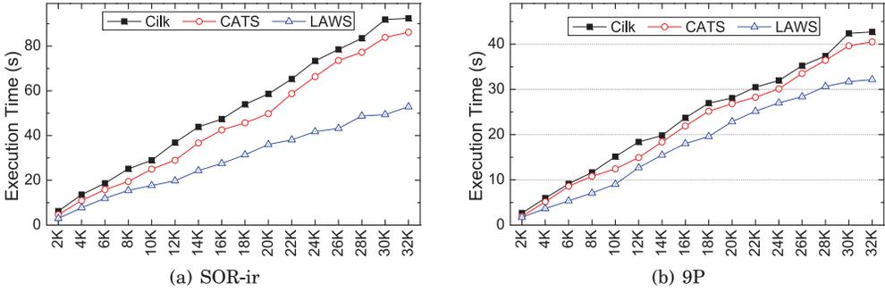
Fig. 10. Performance of SOR-ir and 9P with different input data sizes on the Intel server.
