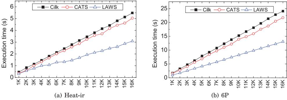
Fig. 9. Performance of Heat-ir and 6P with different input data sizes on the AMD server.
