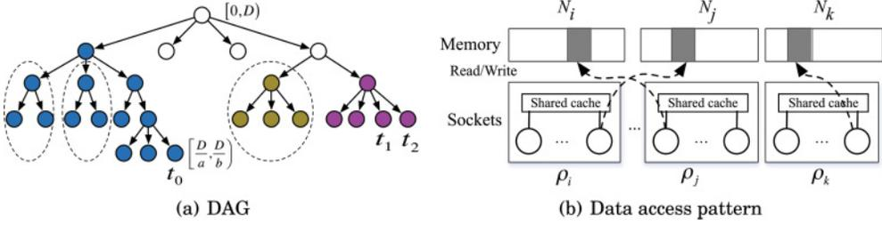
Fig. 2. An example DAG and the data access pattern in traditional work stealing on MSMC architecture.
