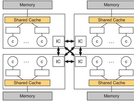
Fig. 1. An example of MSMC architectures that employ NUMA-based memory systems.
