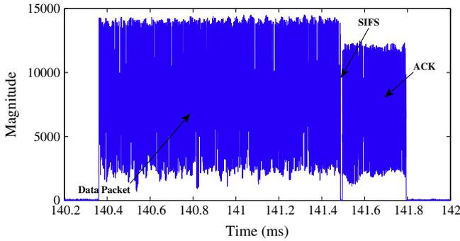
Fig. 2. The SIFS interval between data messages and ACKs can be obtained with a sample rate of 4 MHz.
