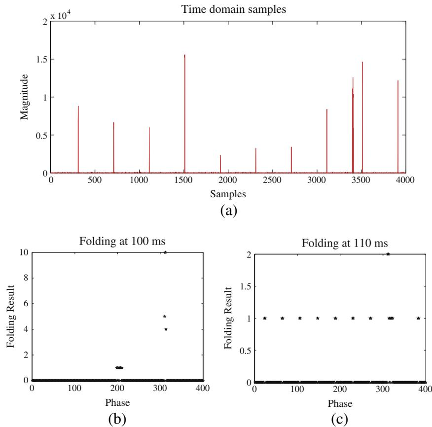
Fig. 8. (a) The magnitude of collected samples in 1 s. (b) The folding result at the correct period. (c) The folding result at the wrong period.
