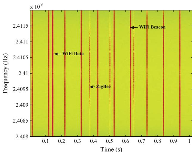
Fig. 5. Spectrogram of the ISM band centered at 2.41 G and spanning 4 MHz.
