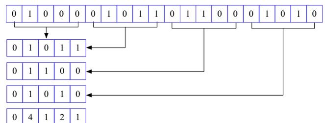
Fig. 6. Operation of Folding Algorithm. In this time series, there is a periodic symbol with period 5 at position 2. After FFA, there is a peak with magnitude 4 at position 2.
