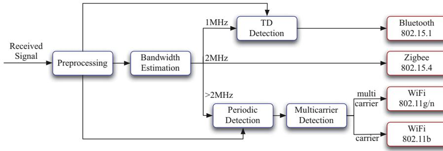
Fig. 4. System block diagram.
