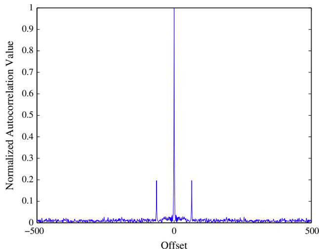
Fig. 9. Autocorrelation result of received OFDM signals.
