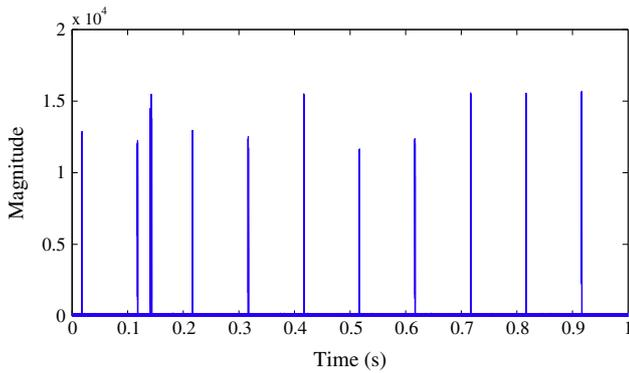
Fig. 3. Magnitude of 802.11 signals collected in 1 s with 4 kHz as its sample rate.
