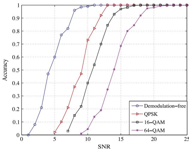
**Fig. 11.** Detection accuracy between demodulation-free and demodulation-dependent method under low SNR.
