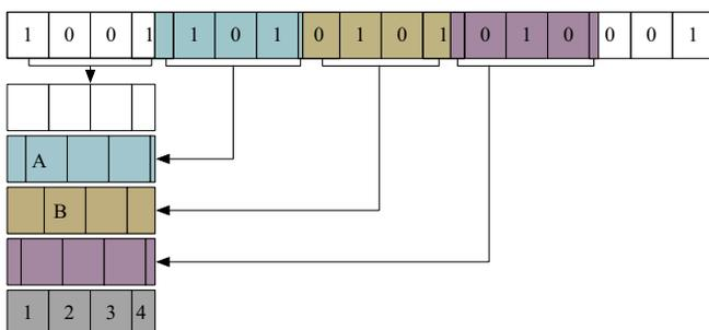
Fig. 7. Operation of Precision-Stable Folding Algorithm. The sequence is folded at a decimal period of 3.6.
